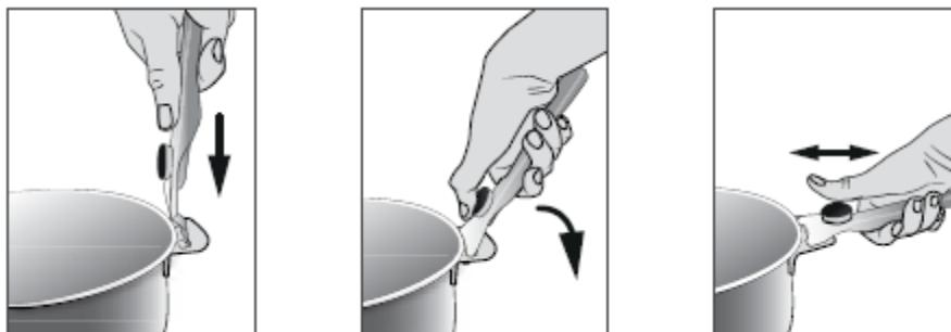
A “click” signals that the handle is correctly in place.
